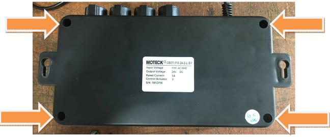
1. Remove the four (4) Phillips head screws from the back of the controller.
