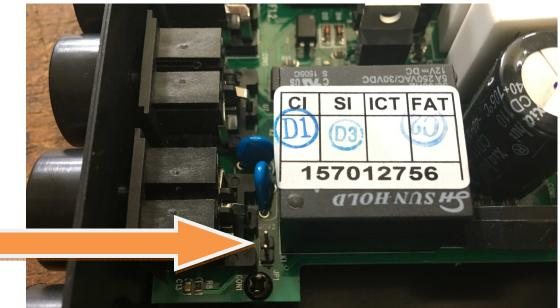
4. Install the jumper using needle nose pliers.
